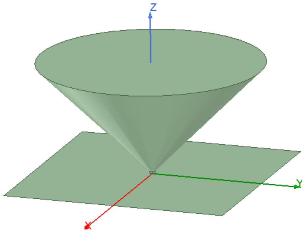
Building this model is straightforward. You need to create a 3D solid cone and two rectangular sheet objects—one to serve as an infinite ground plane and one as a port.
